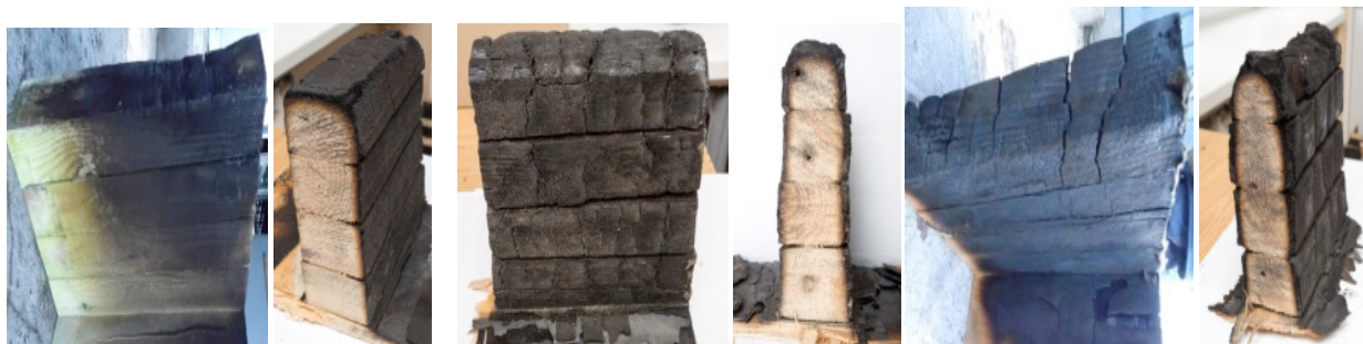
Figure 1 – Photo samples after fire tests.
