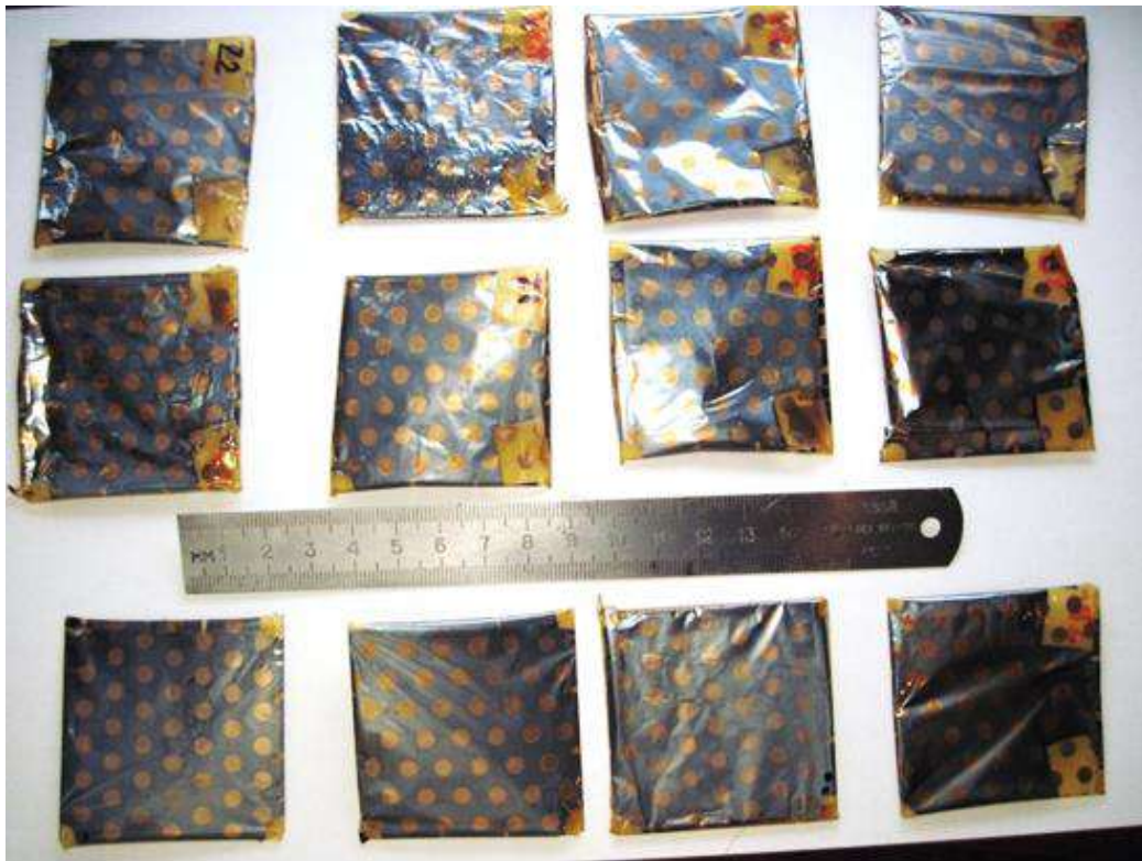
Fig. 1. General view of thin-film ITO/CdS/CdTe/Cu/Au PVC samples.
