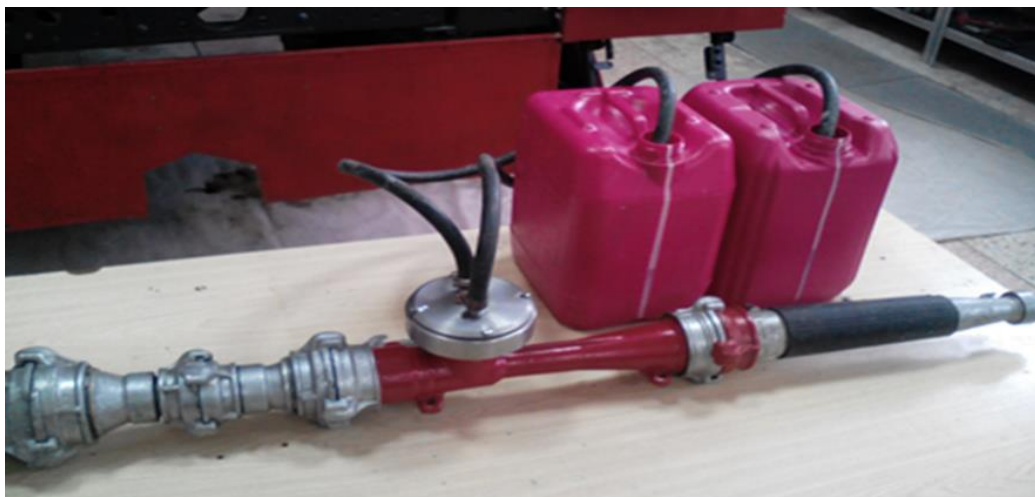
Picture 1. – Appearance of a portable ejector type device for producing a fire extinguishing gel
