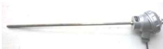
Figure1. TXA-VIII thermocouples (0 to 1100)°C.
