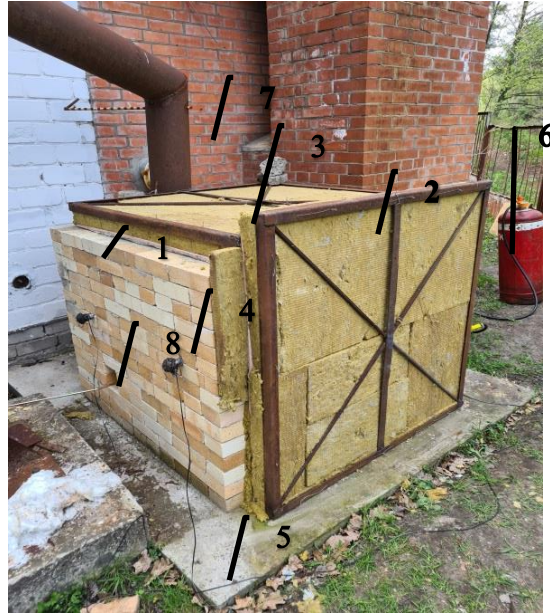
FIGURE 1. Prototype of a compact installation for testing reinforced concrete and reinforced concrete building structures under the thermal effects of fire: 1- n-shaped box; 2-3- removable covers; 4- thermocouple; 5- power floor (foundation); 6- gas installation; 7- chimney for the output of combustion products; 8- hole for installation of burners.
