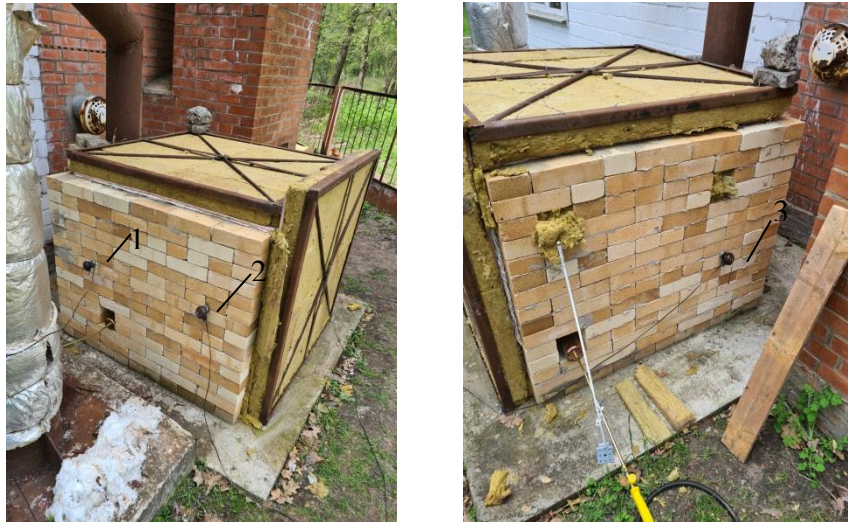
FIGURE 2. The Location of Thermocouples in the Walls of the Test Installation for the Study of Temperature Distribution in the Furnace Chamber: 1-3 – Thermocouples of TCA Eye.
