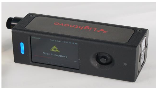
Figure 2. Lightnovo ApS handheld miniRaman spectrometer
