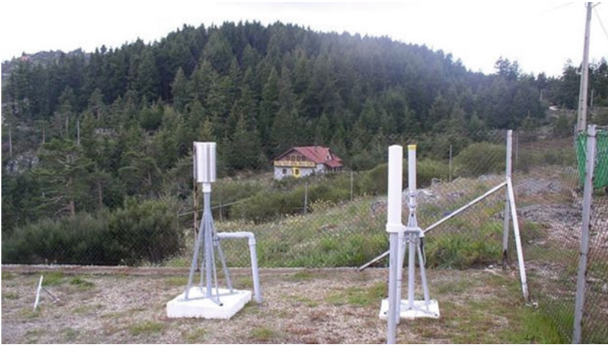
Fig. 8 Automatic station of radiation monitoring [19]
