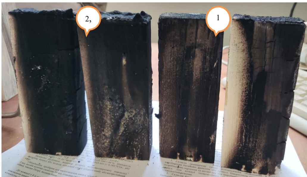
FIGURE 3. The appearance of films of an intumescent organic binder of composite materials for protection against electromagnetic fields after accelerated and firing tests with a film thickness of 0.5 mm (2) and 1 mm (1).
