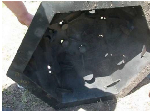
Fig. 5. Protective device inside after explosion.
