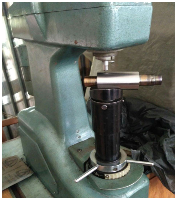
Fig. 2. Rockwell hardness tester measuring the surface hardness of one of the rolls.
