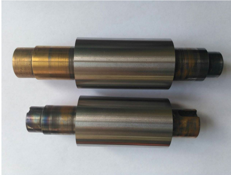
Fig. 1. A pair of rolls (40X steel) that need to be restored to their original performance.
