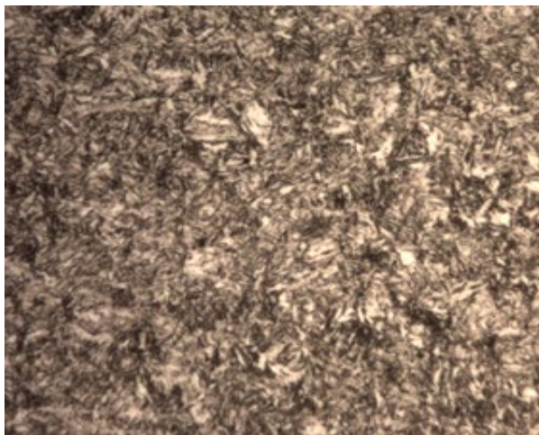
Fig. 4. Microstructure of 40X steel after quenching and cooling in water, \times 500 .
