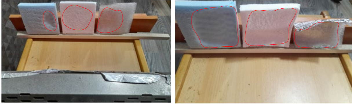
Fig. 3. A view of the specimens of synthetic materials during their thermal decomposition under the thermal radiation
