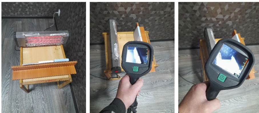
Fig. 2. Measuring the material surface temperature
