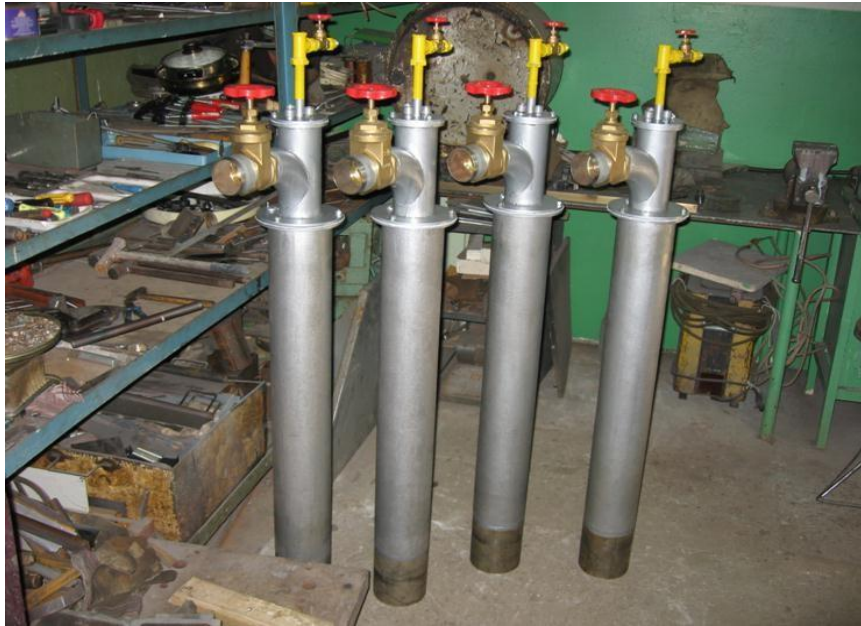
Figure 4. Gas burner devices of the HS series for a shaft furnace
