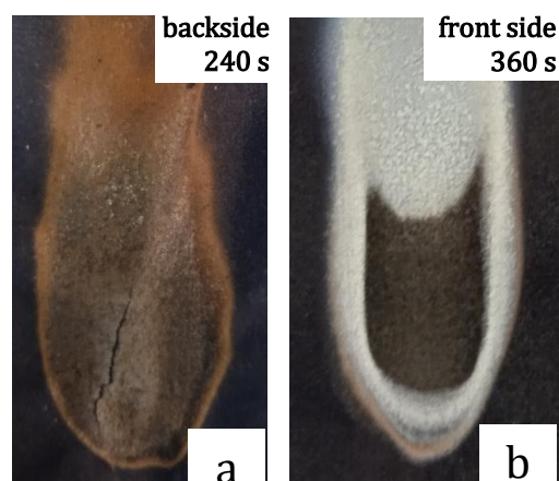
Fig. 3. Photo of samples after tests. Sylgard-184 coating without filler (a) and proposed composition (b)
