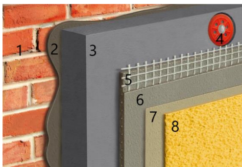
Fig. 1 Facade insulation system components. (1) The foundation of masonry; (2) Mineral glue „Sakret BK“, yield about 5 kg/m 2 ; (3) Gray polystyrene foam „EPS 70“ thickness 180 mm, density 14.0 kg/m 2 ; (4) Plastic studs, yield 4 pcs/m 2 ; (5) Sakret fiberglass mesh, area weight about 160 g m 2 . Manufacturer UAB Sakret LT; (6) Mineral reinforcement plaster „Sakret BAK“, yield about 5 kg/m 2 ; (7) Polymeric primer before decorative plaster Sakret PG yield about 0.25 l/m 2 ; (8) Decorative plaster Sakret SBP, yield about 4 kg/m 2 .
