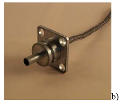
Figure 2. Schematic graphical representation of FOA 013-01 receiver (a): 1 – constantan disk, 2 – receiver housing, 3 – cooling jacket, 4 – wire, 5 – connection socket; (b) photo of FOA 013-01 heat flux receiver.
