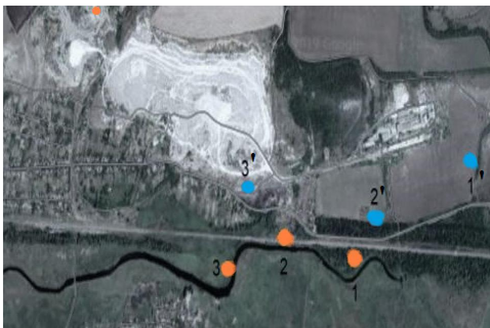
Fig. 1. Soil sampling points in the area of influence of the source of danger were located at a distance of up to 500 m (1'), up to 300 m (2'), up to 700 m (3') from the source of danger; water sampling points from the river were taken at a distance of 5 km downstream (1), 3 km, (2) and 5 km upstream (3) from the source of danger.
