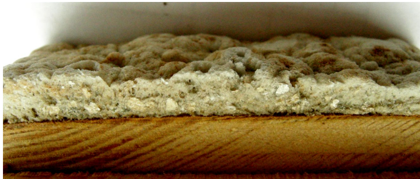
Fig. 4. Cut type of fire retardant coating
