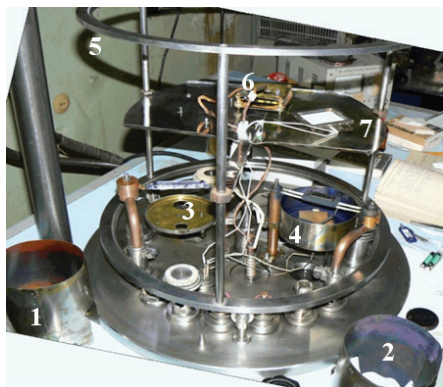
Fig. 1. The internal installation system for spraying CdS and CdTe: 1, 2 – screens, 3 – evaporator of powdered cadmium telluride; 4 – evaporator of powdered cadmium sulfide; 5 – carousel, 6 – substrate heater, 7 – substrate holder
