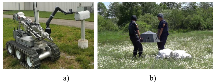
Figure 1. Examples of bomb disposal devices: a) remotely controlled bomb disposal robot Andros Wolverine 6X6 (source [27]), and b) a prototype of a smart cone device from the National University of Civil Defence of Ukraine, Ukraine (courtesy of Yevhen Stetsiuk).
