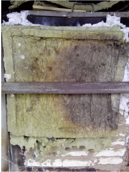
Fig. 4. View of the test sample from the non-heating surface of the steel plate
